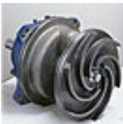
**Inspection of pump shaft or bearings is easily accomplished without disturbing pump casing or piping by removing rotating assembly. Simply remove four bolts from the back of the pump and the assembly slides out.**
