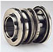
**Exclusive double-floating, self-aligning, oil lubricated mechanical cartridge seal with stationary and rotating face of silicon carbide or tungsten titanium carbide is specifically designed for abrasive industrial service. Fluorocarbon and PTFE elastomers are also available.**
