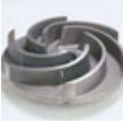
**Multi-vane, high efficiency solids handling impeller constructed of ductile iron. The impeller will handle up to 1 1/4" diameter solids.**
