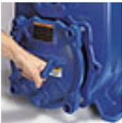
**The removable cover plate with "easy-grip" handle and pusher bolt capability provides quick and easy access to the pump interior without disconnecting piping. Clogs can be removed and the pump can be returned to service in minutes. Impeller, seal, wearplate and flap valve can also be accessed through cover plate opening for inspection or service.**
